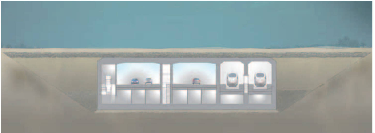
Figure 5. The Fehmarnbelt tunnel will be constructed from 79 standard elements each 217 m long and 10 shorter special elements to be located every 1.8 km.
